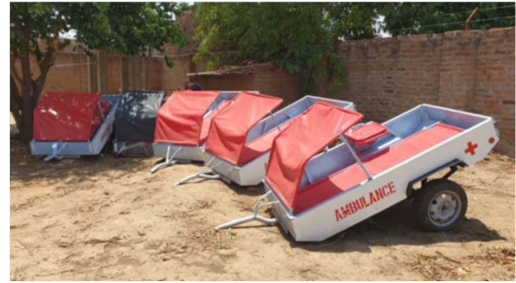
October 2020 Eric Kroner - Chad Team, a rear-motorcycle ambulance cart designed by Scott and a short-term visitor Patrick with local resources and labor
